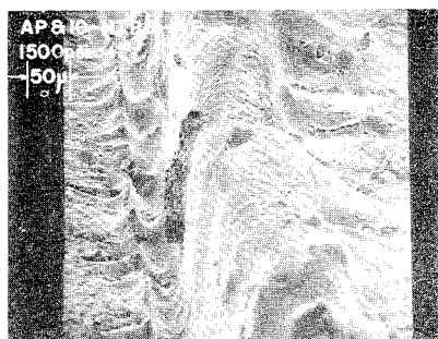
Fig. 3 AP and ferric oxide-HTPB-AP sandwich quenched at 1500 psia ( \times 177 ).
